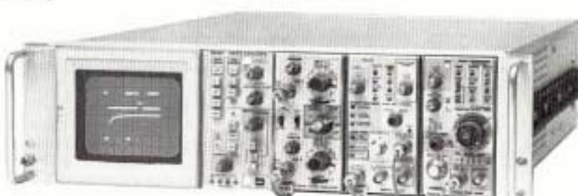
The 7633 and 7623A require only 5.25 in. of rack height in a standard 19 in. rack. They are fan cooled and come complete with slide-out chassis tracks.
